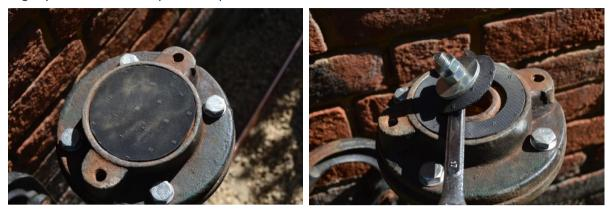
Having ordered a new bucket/valve from Robinson & Sons, it was obvious that the operating rod (also threaded to M10 x 1.5) was too long for the barrel, and we would have to fabricate a new linkage in any event. A yoke was made up from flat steel stripwith a hole at the top for the operating
