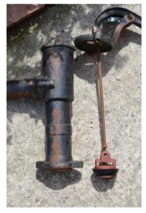
rod. The rod was measured up and shortened with a hacksaw, with the intention of simply re-threading the end with an M10 die. Again, there were problems; the rod was not 10mm, or anything close, and it was proving impossible to get the die started. Without access to a lathe to turn the rod down to the correct diameter, I first re-threaded it with an oversize imperial die, and then recut the threads to
